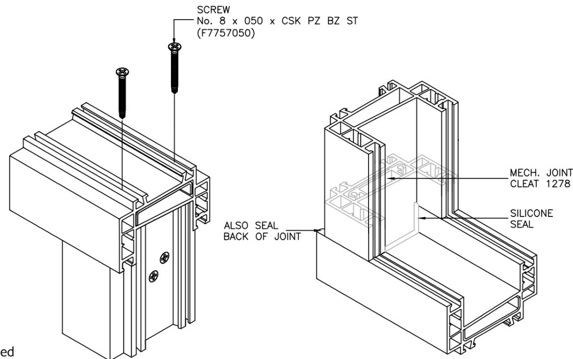
**NOTE:** Outer-frame supplied fully assembled as standard unless otherwise specified
