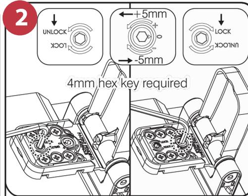
**2** To adjust lateral position, first turn the unlock screw a 1/4 turn. Then use the adjustment screw to adjust up to 5mm in either direction. Finally tighten lock screw.
