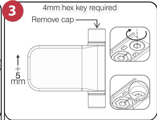
**3** Height adjustment: Using a 4mm hex key turn the screw down to lift the hinge by up to 5mm.
