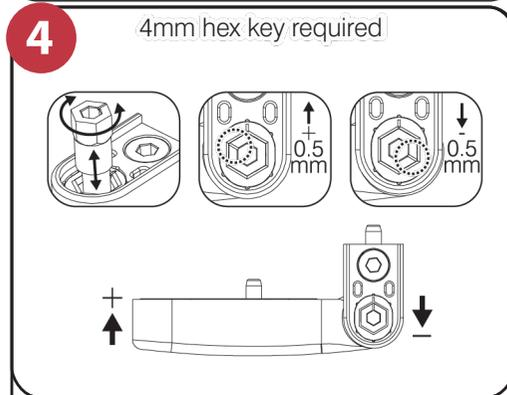
**4** Compression adjustment: Push out hinge pin and turn to alter compression.
