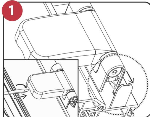
**1** To release cover remove security screw from under the hinge and then insert 5mm blade screwdriver and twist. Use small blade screw driver to release cover caps.
