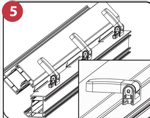
**5** The sash can be removed and fitted when in an open position by lifting or lowering the sash assembly onto the frame datum.
