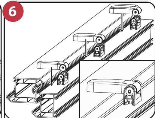
**6** Alternatively the sash can be removed and fitted in the closed position by removing the security screws and hinges pins and then lifting the sash off the frame part.
