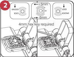
To adjust lateral position, first turn the unlock screw a 1/4 turn. Then use the adjustment screw to adjust up to 5mm in either direction. Finally tighten lock screw.
