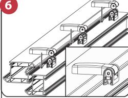
Alternatively the sash can be removed and fitted in the closed position by removing the security screws and hinges pins and then lifting the sash off the frame part.
