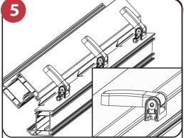
The sash can be removed and fitted when in an open position by lifting or lowering the sash assembly onto the frame datum.
