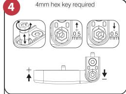
Compression adjustment: Push out hinge pin and turn to alter compression.
