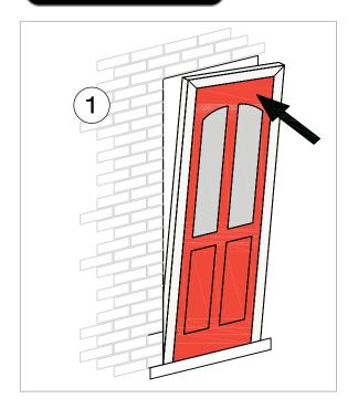
2. Hold frame into position using appropriate size wedge packers.
