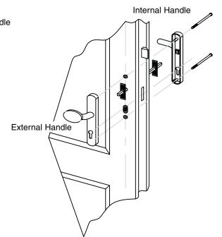
**NB:** When the door has been fixed into position the operation of he door opening and locking mechanism must be checked to ensure uniform contact with weatherseals and correct function of handle/lock.
