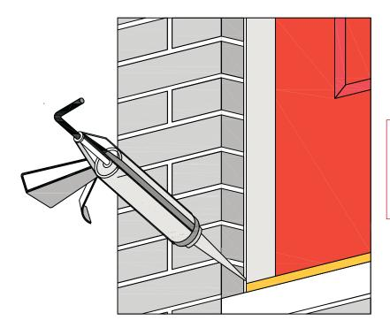
**NB:** Care must be taken to ensure that the drainage slots are not blocked when sealing around the aluminium Low Threshold.
