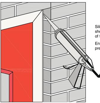
Silicone sealant or similar suitable product should be used to seal around the perimeter of the newly installed composite door frame.
