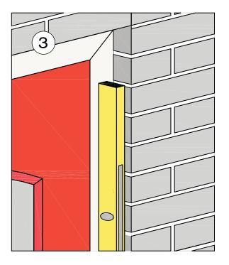
1. Offer complete door unit into brickwork opening.
