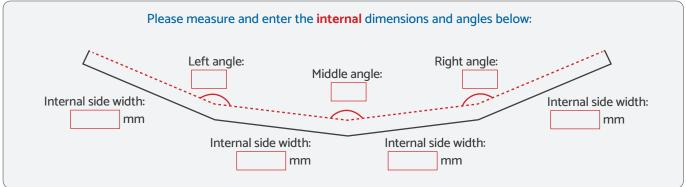
**Widths & Angles** - Once you have determined the internal width measurements, enter these dimensions into the provided boxes. Note you are measuring from the corner of the existing frame to the centre of where the frames join together. I.e between the existing bay poles or bay corner angles.
